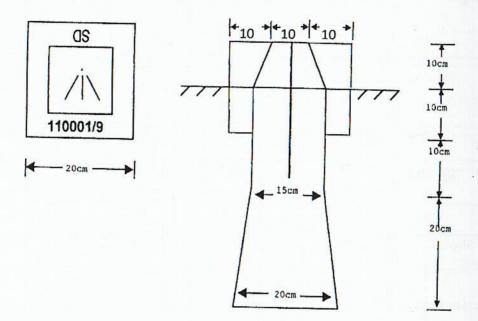
Diameter of the rod is 3mm and length 30 cm
