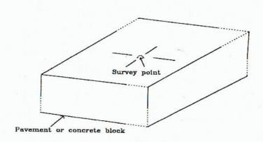
Description :- Brass bolt on pavement, concrete slab etc.
