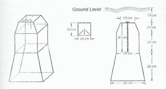
Description: Length of brass bolt -30m, Diameter of the brass bolt -3mm.
