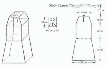
Description: Length of brass bolt -65 mm, Diameter of the brass bolt -12 mm
